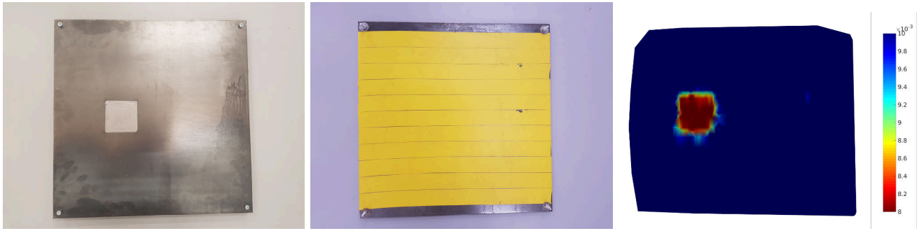
Fig. 13. 10mm thick mild steel sample used for system validation experiments. Left: back side with a 2mm deep slot, middle: front side with yellow coating applied, right: thickness scan produced using our system in millimetres ( 10^{-3}m ).
